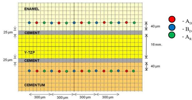
**Figure 2** An illustration showing Vicker microhardness obtained at a 40-micron level on the enamel above enamel-resin cement junction and on the cementum below cementum-resin cement junction (five locations each and with a 100-micron distance apart) before demineralization ( $B_D$ ), after demineralization ( $A_D$ ), and after remineralization ( $A_R$ )
