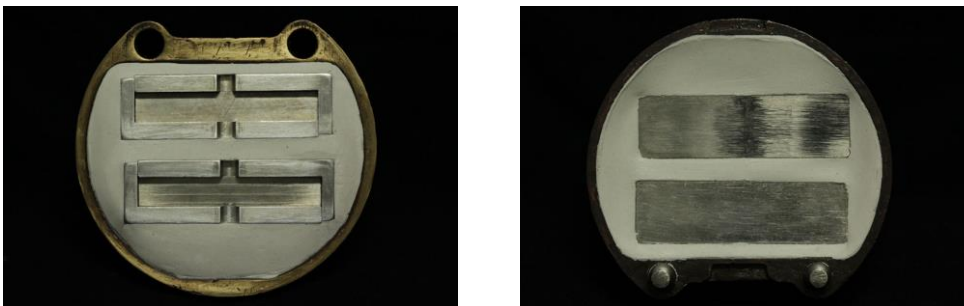
Figure 2 Flasking for heat polymerized acrylic resin with compression molding technique A. Lower half flask B. Upper half flask
