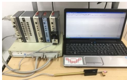
Figure 1 A force transducer (UFI 1030, USA) connected to Biopac system (MP100, USA) with a probe size of 1 cm 2 .
