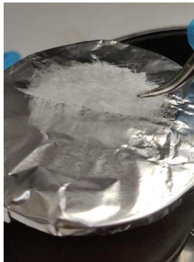
**Figure 7** The electrospun PCL fibers on fiber collector
