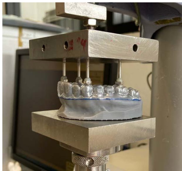
Figure 2 Installation of the sample to the universal testing machine.
