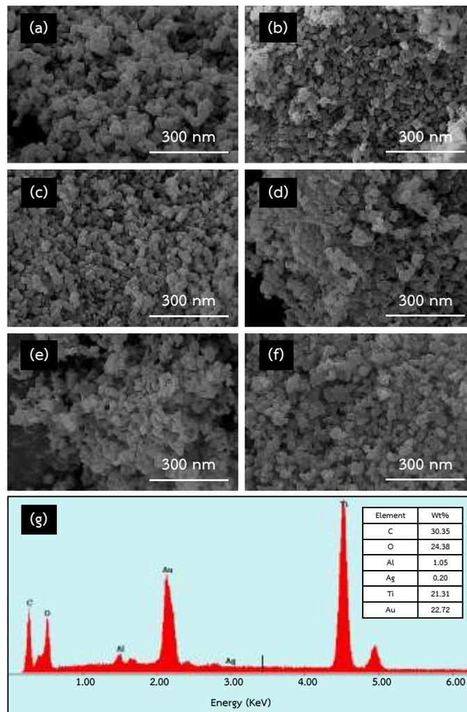
**Figure 6** SEM images of (a) TiO<sub>2</sub>, (b-f) Ag/TiO<sub>2</sub> at different concentration and (g) EDX spectra of Ag/TiO<sub>2</sub>.
