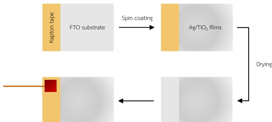
**Figure 2** Electrode preparation of Ag/TiO<sub>2</sub> films
