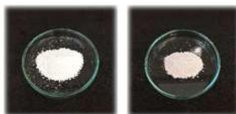
**Figure 1** TiO<sub>2</sub> and Ag/TiO<sub>2</sub> samples by ball milling process.
