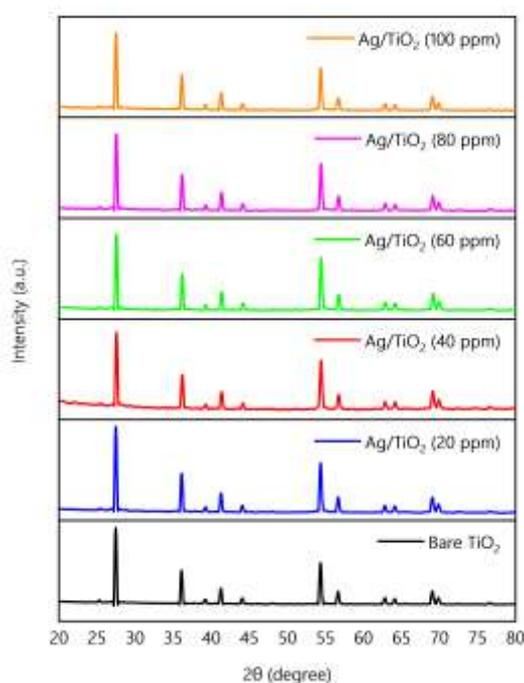
Figure 3 XRD patterns of TiO<sub>2</sub> and Ag/TiO<sub>2</sub> nanoparticles.
