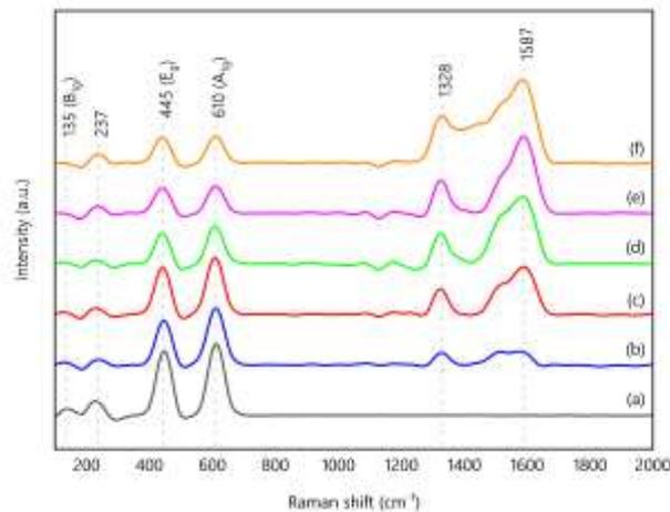
**Figure 4** Raman spectra of (a) bare TiO<sub>2</sub> and (b-f) Ag/TiO<sub>2</sub> nanoparticles
