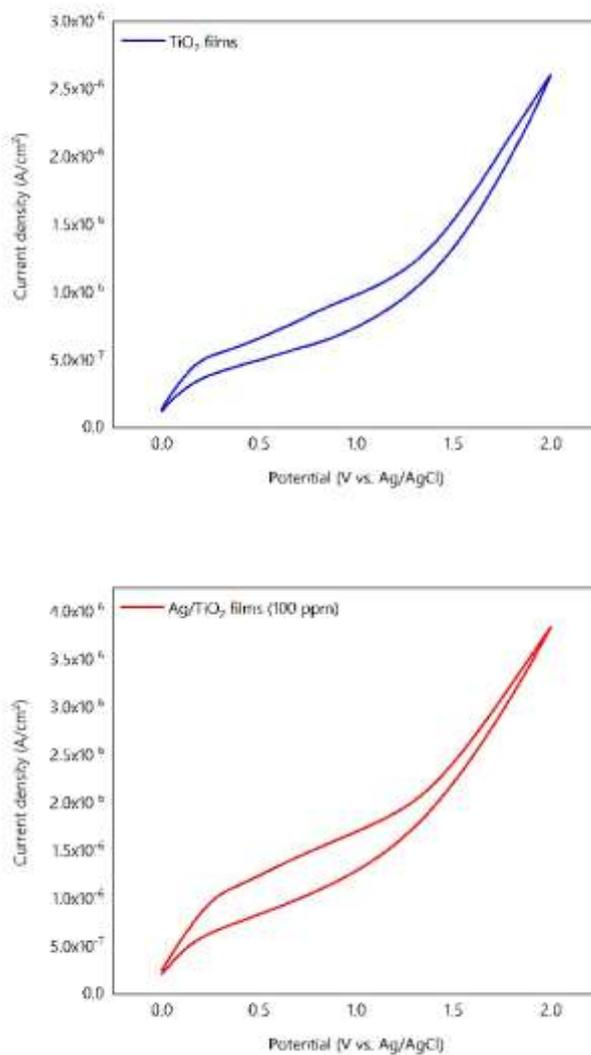
**Figure 8** CV curves of the samples: (a) TiO<sub>2</sub> films and (b) Ag/TiO<sub>2</sub> films.
