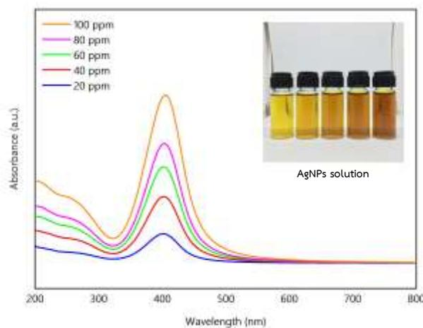
**Figure 5** UV-Vis absorption spectra of AgNPs.
