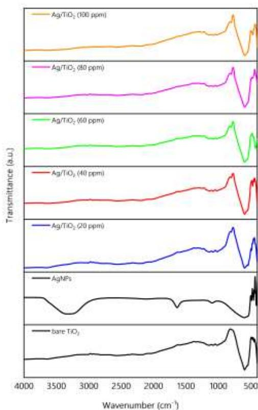
Figure 7 FTIR spectra of TiO<sub>2</sub> and Ag/TiO<sub>2</sub> nanoparticles.
